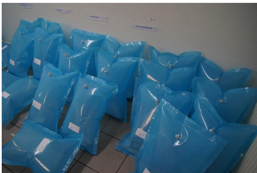
Bags filled with the sample gases for the test.
